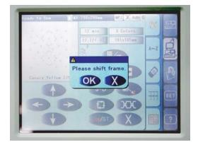
Detach the hoop from the machine and shift the frame to position 2 and reattach to machine.
