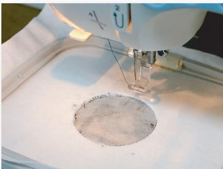
Slide dissolving fabric under hoop to completely cover cutout hole.
