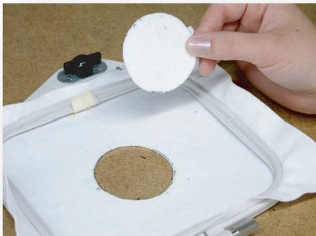
Remove cutout hole and reattach hoop to the machine.
