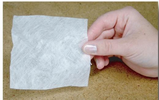
Shown - sample of dissolving fabric, (e.g. H2O Gone, Aquamagic). It is not recommended that dissolving plastic be used, (e.g. Solvy).
