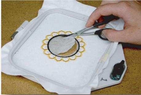
Remove hoop from machine and cut away excess dissolving fabric.
