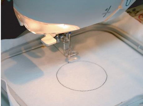
Hoop desired fabric and slide one layer of lightweight tearaway underneath. Sew design until cutline stop.
